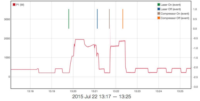
Fig. 9. Identifying large shop loads. The cross correlator identifies transients of machines in the shop that might interfere with the 3-D printer.
